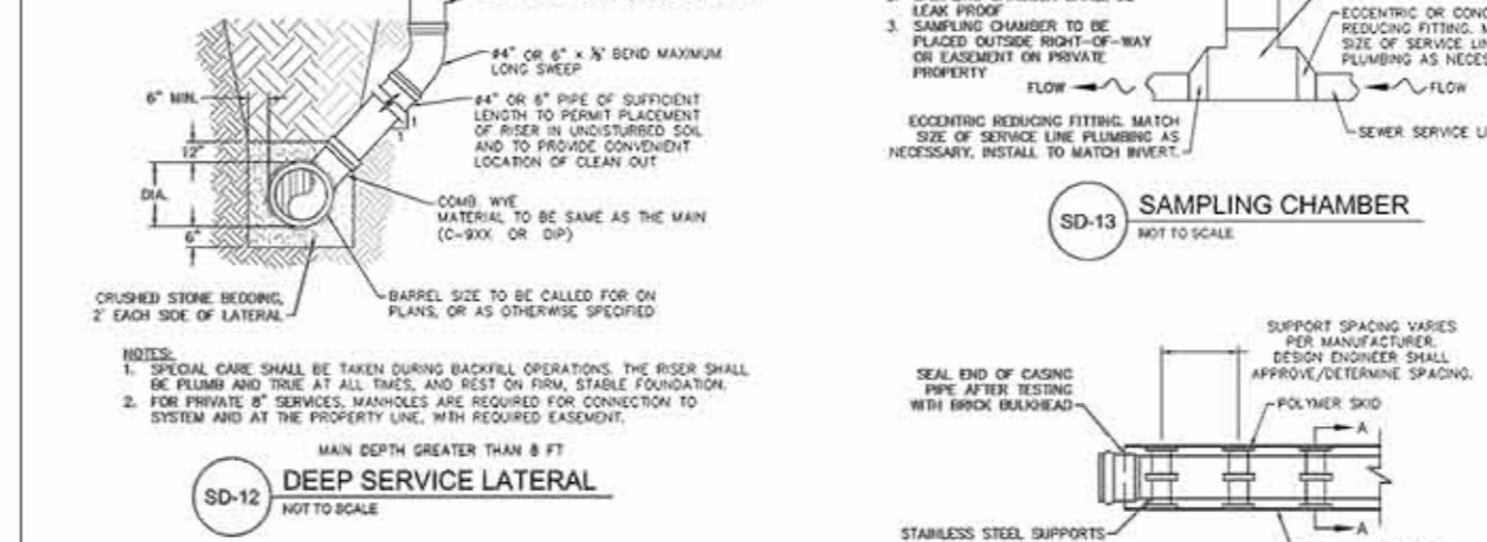
SD-13 SAMPLING CHAMBER NOT TO SCALE
